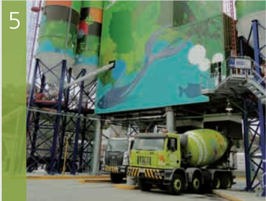
collection system can store up to 100,000 liters of water that can be used to produce the concrete and for other production activities. The admixtures system supplies 9 types of different materials that can produce a wide range of concrete. Aware of the importance of this plant for the company and the city, on its 35th anniversary Concretos Moctezuma decided to decorate all the facades of the buildings on the site, including the silos and the tower,
